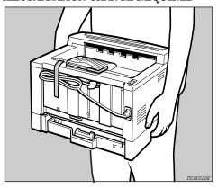
Remove the four pieces of adhesive tape from the printer as shown in the illustration. ILLUSATRATION CHANGE REQUIRED
