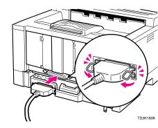
Attach the other end of the interface cable to the interface connector of the computer. Secure the
