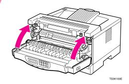
$\Box$  Do not close the front cover with force. If you cannot close the cover easily, pull out the toner cartridge from the printer and insert it again. After that, close the front cover again.
